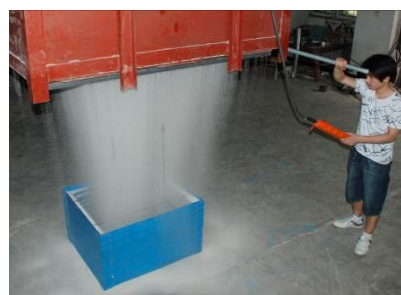
图2 分层砂雨法制备模拟地基 Fig.2 Model foundation preparation with sand rain
