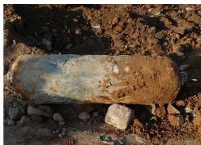
图1 多重防腐囊式扩体锚杆(CJY-KT 锚杆) Fig.1 Multiple anti-corrosion capsule-shaped underreamed ground anchor(CJY-KT anchor)
